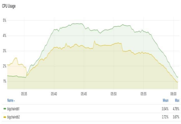
Figure 4. 1k inserts CPU usage BigchainDB node1&2
