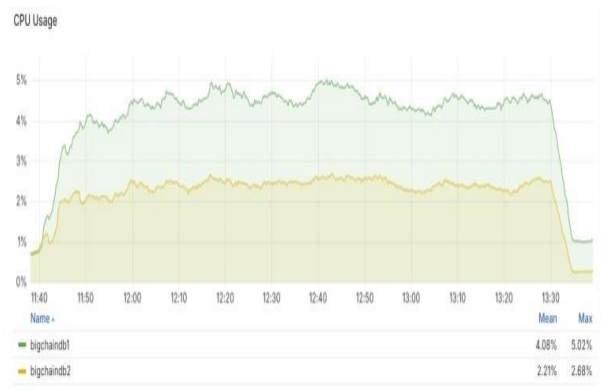
Figure 8. 5K inserts CPU usage BigchainDB node1&2
